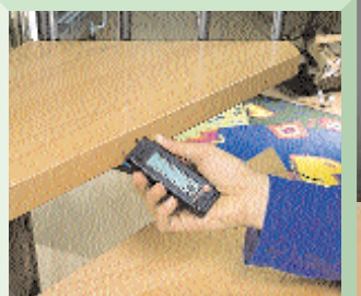
Moisture monitoring in building materials
