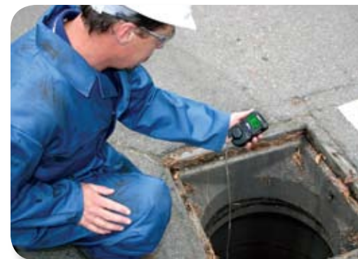
QRAE II being used with built-in pump for a confined space entry
